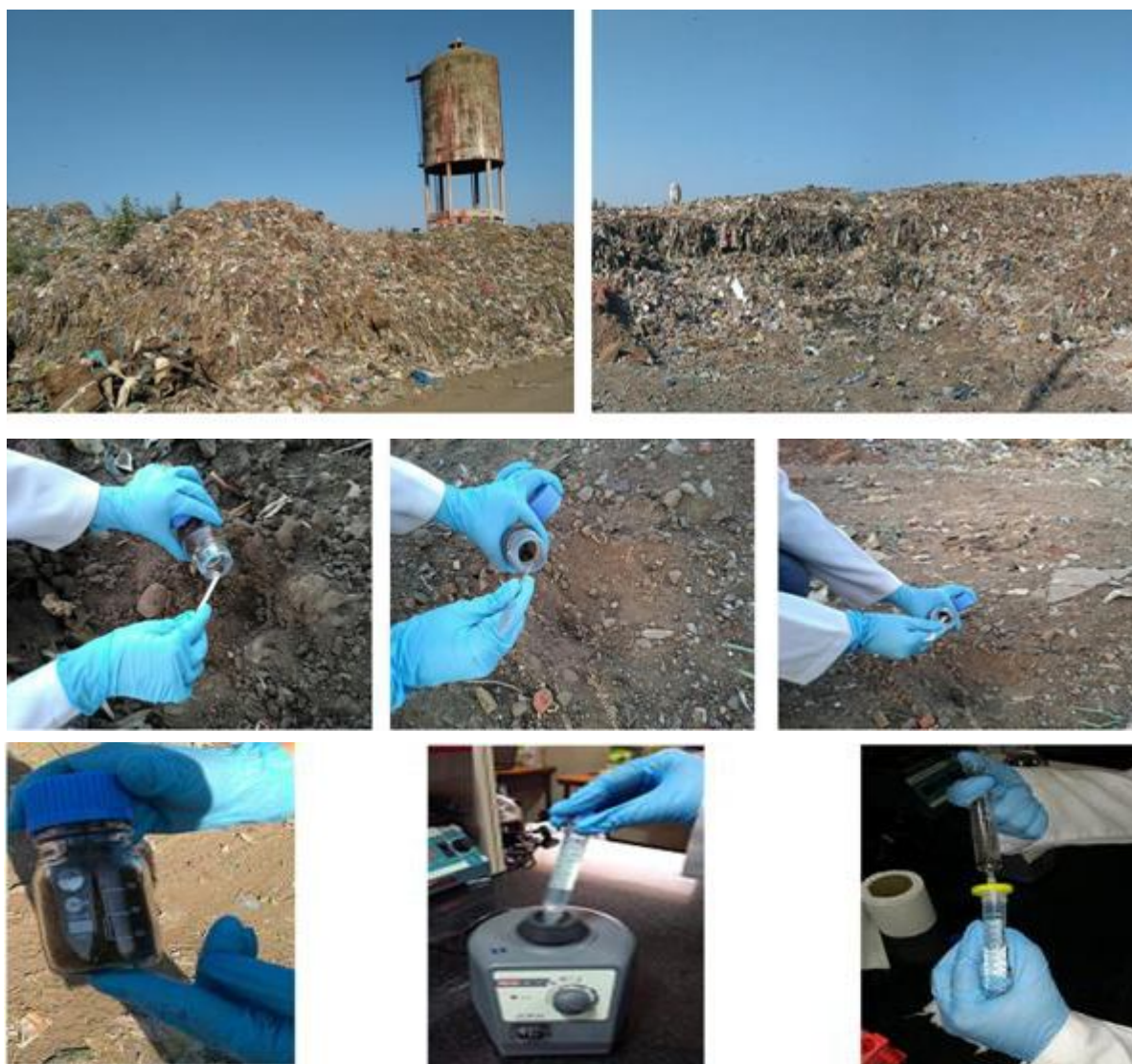
Fig- 43 : Collection of soil samples from Bhanupur landfill area and preparation of leachate in the laboratory
